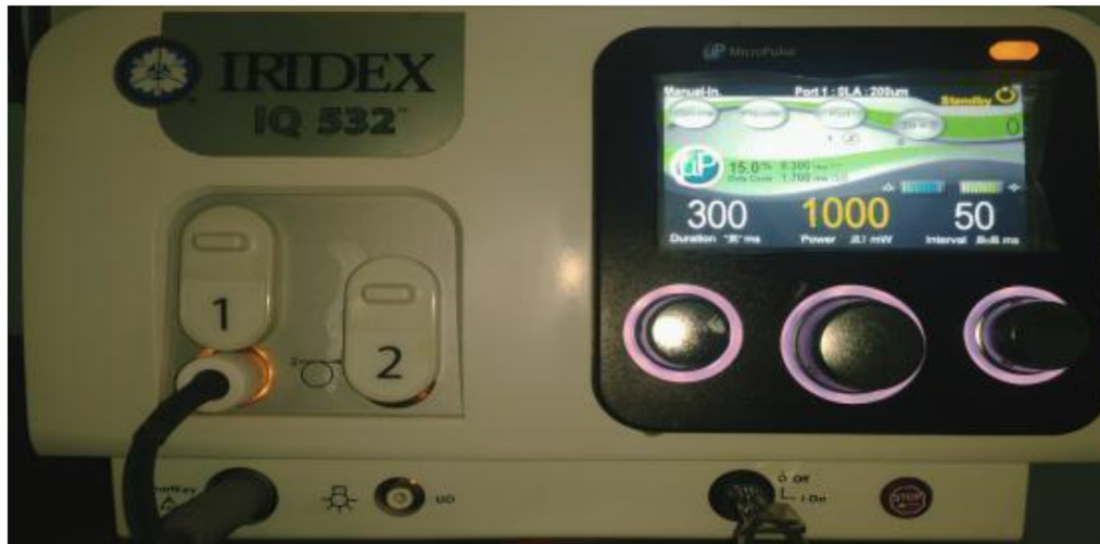
Fig. 2. Iridex IQ 532 argon laser apparatus subthreshold micro pulse: showing parameters of laser used in MLT procedure.
