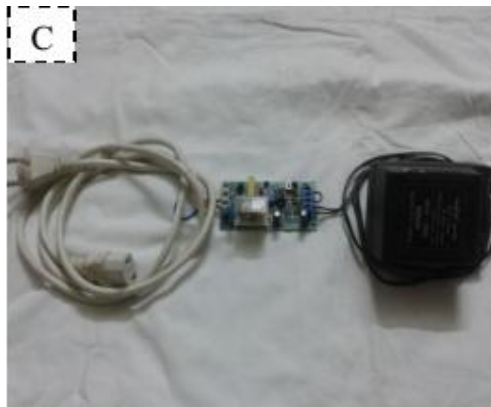
Fig. 2: The VAC machine, (A) the suction machine, (B) the pressure adjusted in bar, (C) the electrical timer circuit.
