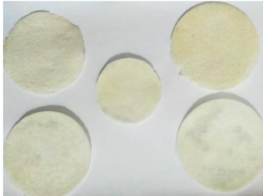
Fig 1: Polycaprolactone scaffold after fabrication
